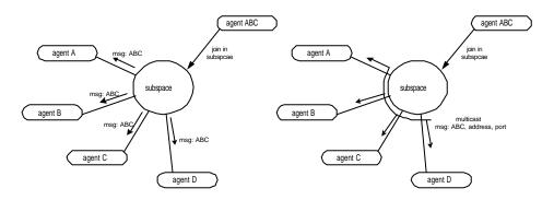
Figure 3-12 unicast vs. multicast entry message
