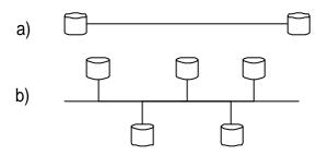
Figure 2-3 Direct links: a) point-to-point; b) multiple access
