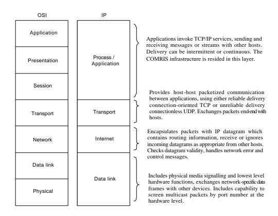
Figure 2-4 Correspondence between OSI and IP protocol layer model
