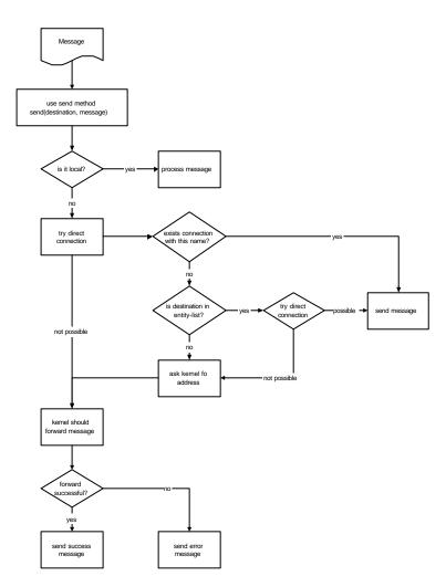
Figure 4-2 Message flow diagram for direct connetion
