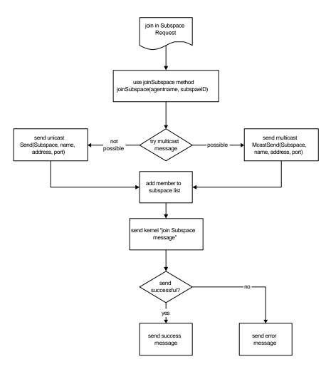
Figure 4-3 Flow diagram for address multicast
