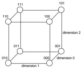
Figure 3-9 A 3-dimesional hypercube
