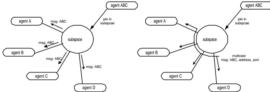
Figure 3-12 unicast vs. multicast entry message
