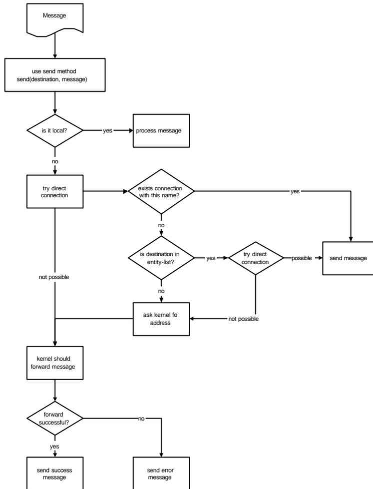
Figure 4-2 Message flow diagram for direct connction
