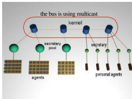
Figure 3-5 Example for a bus topology
