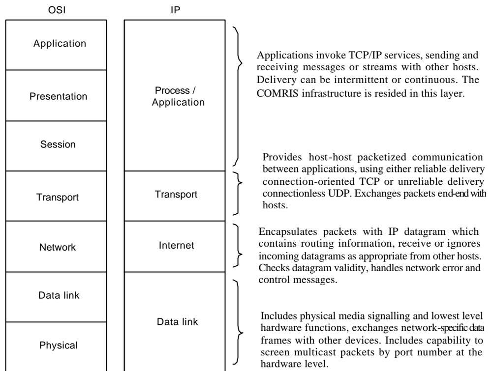
Figure 2-4 Correspondence between OSI and IP protocol layer model
