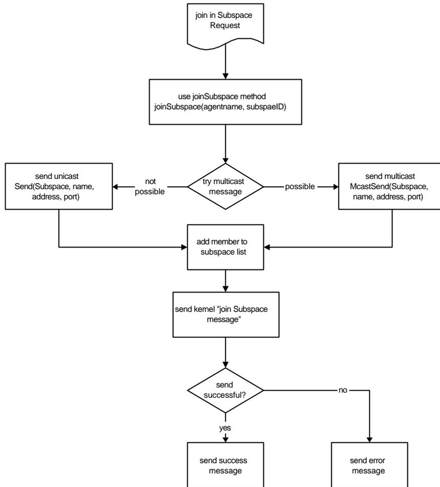
Figure 4-3 Flow diagram for address multicast
