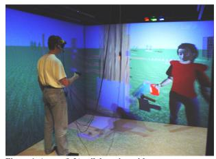
Figure 1. A user (left) collaborating with a remote user (represented by avatar, right) via linked walk-in displays.
